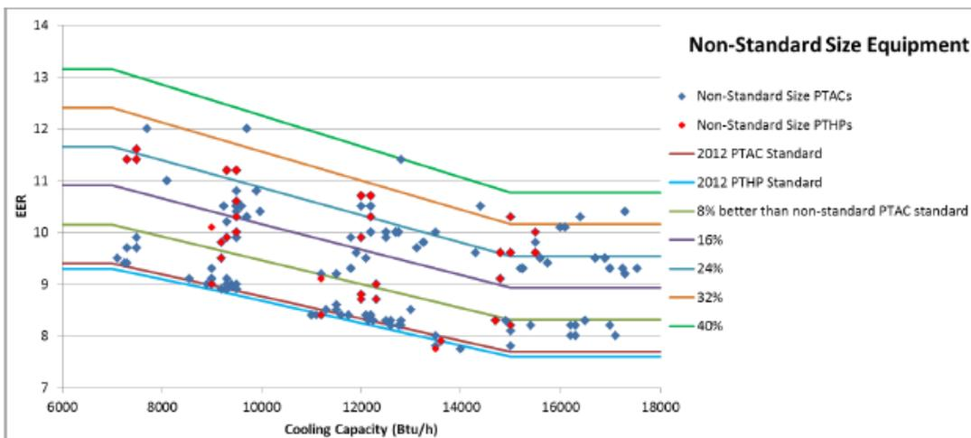
As can be seen in the graphs above, the proposed efficiency levels for the analysis capture the range of efficiencies of currently available PTACs and PTHPs. However, the maximum available efficiency level is not necessarily equivalent to the maximum technologically feasible level. DOE must evaluate a true “max tech” level, which we expect would be higher than the efficiency level of the most-efficient commercially available products.
